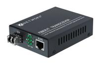
This Fiber Transceiver / Media Converter is designed to convert data signal between 10/100/1000Base-T and 1000Base-LX Gigabit Ethernet. Maximum transmission distance 20 kilometers over duplex single-mode fiber (9/125 micron) @ 1310nm. Duplex LC Connector.
