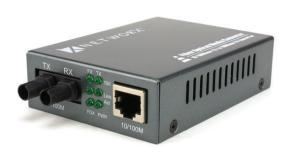
**Extended Transmission Distance:** Converts signals from 10/100Base-TX to 100Base-FX, extending transmission distances up to 120km over fiber optic cable, significantly beyond the 100m limit of copper cables.
