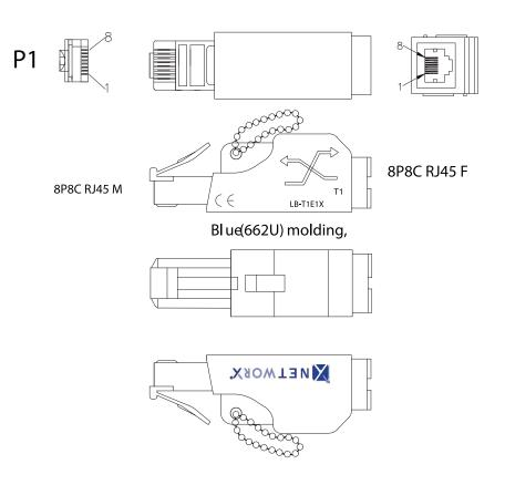
Easy Conversion: Transforms any standard Ethernet cable into a crossover cable, enabling direct communication between similar devices such as routers or switches.
